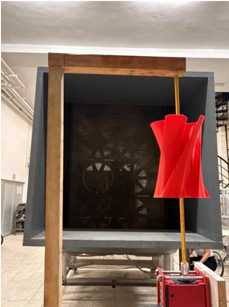
Fig. 6. Model 3 - The experimental view of the helical, models in front of the wind turbine.
