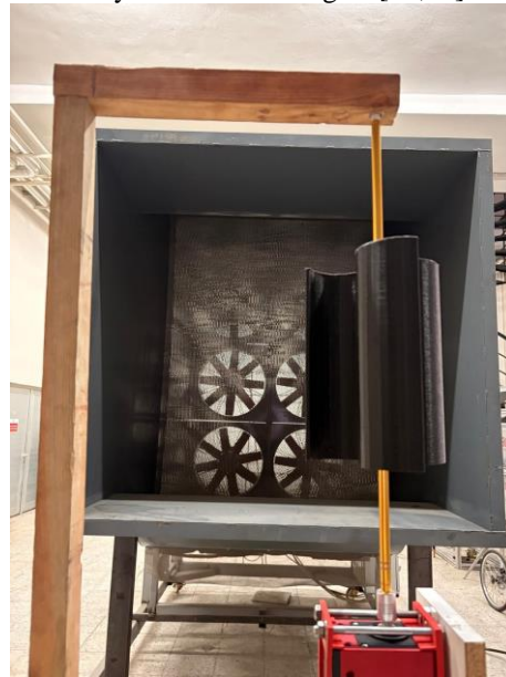
Fig. 4. Model 1 - The experimental view of the classical, blade models in front of the wind turbine
