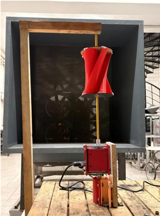
Fig. 7. Model 4 - The experimental view of the helical, blade models in front of the wind turbine
