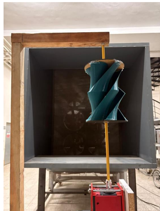
Fig. 9. Model 6 - The experimental view of the hybrid/optimized blade models in front of the wind turbine
