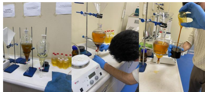
Fig.12 Sedimentation Process (in the separatory funnel)
