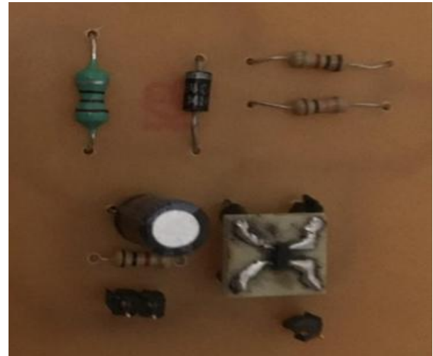
Figure 13. The picture of the proposed buck converter with the MIC94030 MOSFET on PCB.
