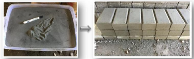
Figure 8. Processed waste tea ash and fresh blocks (adapted from [32])
