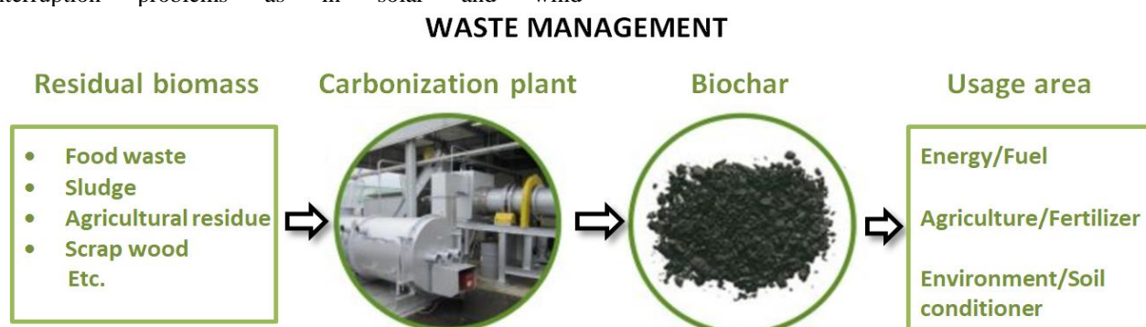
Figure 1. Converting organic waste into biochar and used in different areas (adapted from [5])
